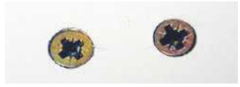
▲ The rival screw on the left shows crushing around the perimeter of the head
